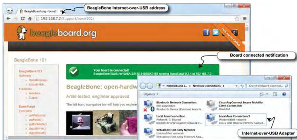
Figure 2-2: Windows Network Connections with Internet-over-USB connection LAN 9, and a web browser connection
