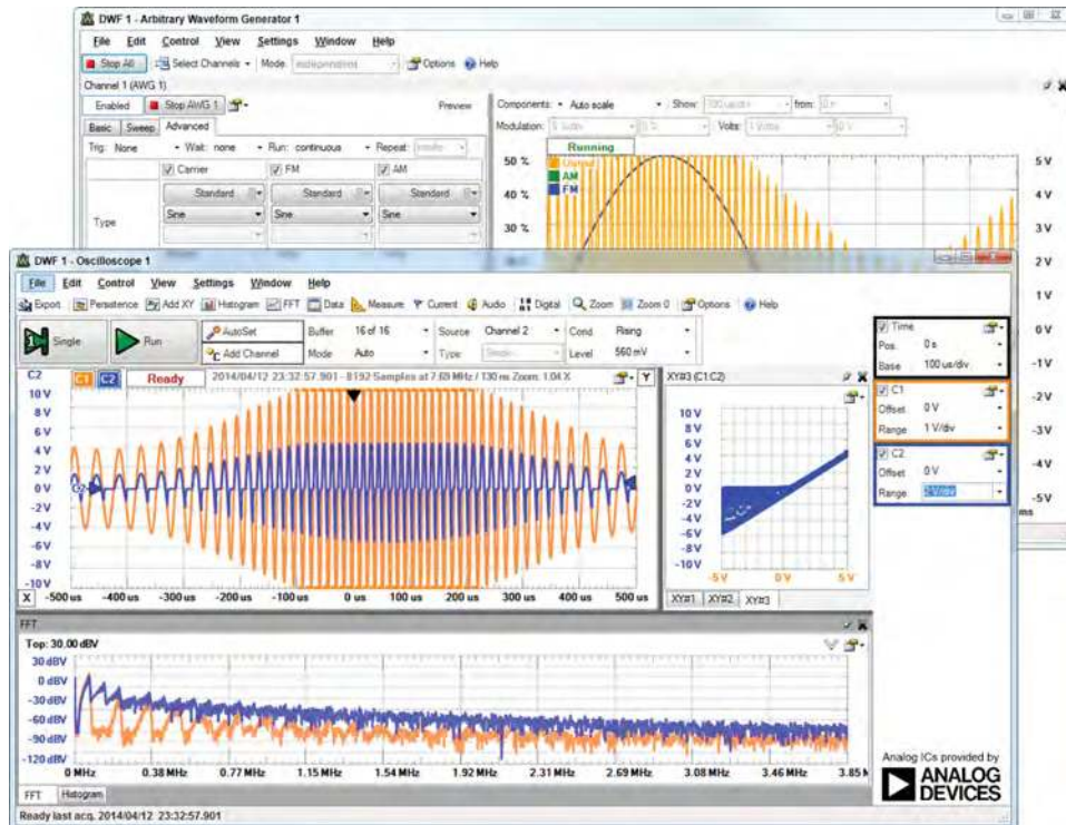
Figure 4-1: The Waveforms application generating a signal and displaying the response from the physical circuit
