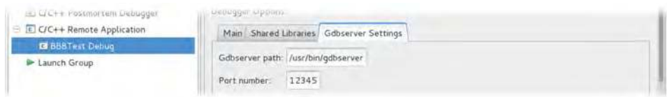
Figure 7-9: Setting the BBB gdbserver port
