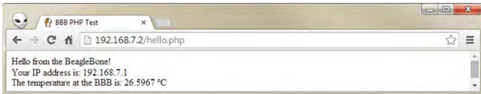
Figure 10-6: A PHP temperature sensor
