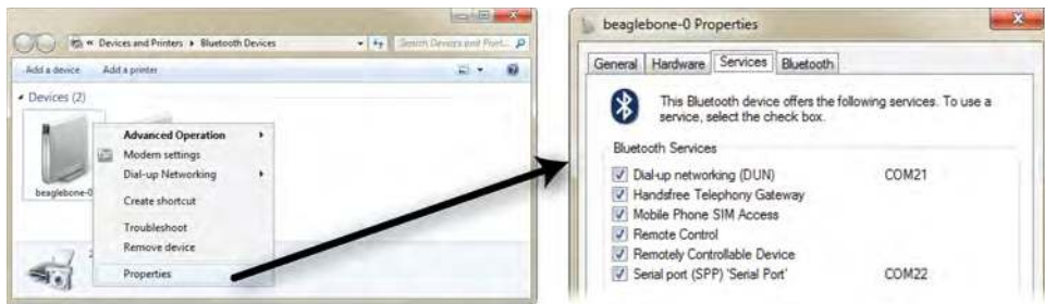
Figure 9-24: Windows connecting to the BeagleBone using an on-board Bluetooth interface
